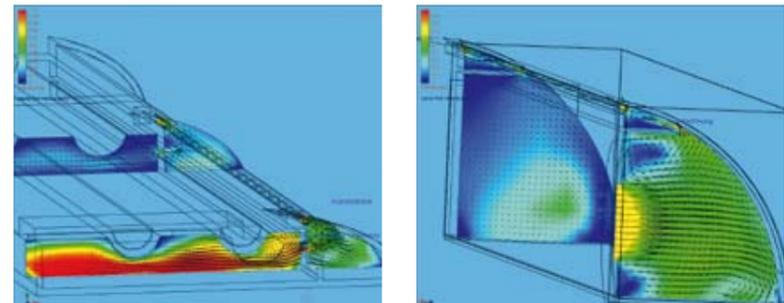
EN 14175 has defined significantly stricter criteria for flow technology in fume cupboards. In particular, the new robustness test defines high requirements for the containment values of fume cupboards. Due to the optimised flow in our new fume cupboards, now even less extract air is necessary to ensure safe operation.
