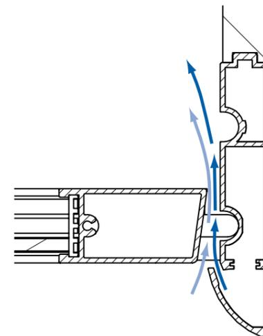
**Cross section through sash and side post.**
